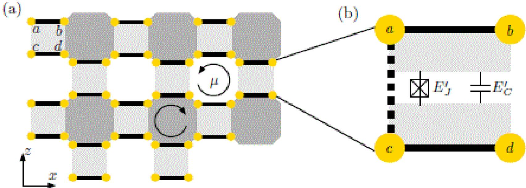
**Light-grey areas** are superconducting (SC) islands, each with two InSb nanowires on top at the end of which are Majorana bound states: 4 Majorana fermions (**in yellow**), representing a single qubit. Tunneling coupling of strength  $\lambda$  for Majorana fermions between islands.
