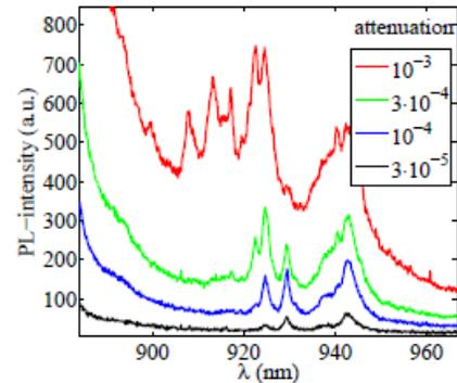
Figure 1: Typical spectra of an InAs quantum dot excited with a laser at 780nm wavelength. The excitation of such high energy causes recombination not only in the quantum dots (between 900 and 960 nm) but also from higher energy states in thin layer of InAs (so called wetting layer) seen here for wavelengths shorter than 900 nm and especially at lower attenuation of the laser beam. This signal can be removed by excitation with laser emitting at 900 nm or longer wavelength.
