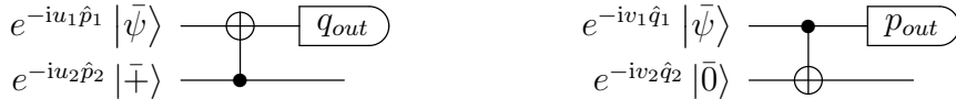
Figure 3.4: Circuits for Steane error corrections via 1-bit teleportation. Left circuit corrects errors in the \hat{q} quadrature. After the CNOT gate we measure the data qubit in the \hat{q} quadrature with outcome q_{out} = u_1 + u_2 + n\sqrt{\pi}, n \in \mathbb{Z} . Based on q_{out} , we need to decide the state of data qubit after measurement, i.e. whether q_{out} is closer to an even multiple of \sqrt{\pi} or closer to an odd multiple. If it's in |0\rangle , the ancilla will be left in state |\bar{\psi}\rangle or with shift error u_2 and v_1 + v_2 , otherwise there would be a logical error. The analysis for the left circuit which corrects errors in the \hat{p} quadrature is the same.
