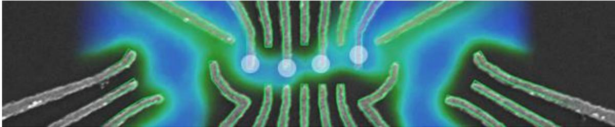
**Fig. 1** Top view of a GaAs sample used in our group, which confines four electrons in two double quantum dots. By applying high-frequency electrical voltage pulses to the grey metal gates, the quantum mechanical state of the left and right qubit can be manipulated individually with very high accuracy. The electron density obtained from simulations is shown in blue.
