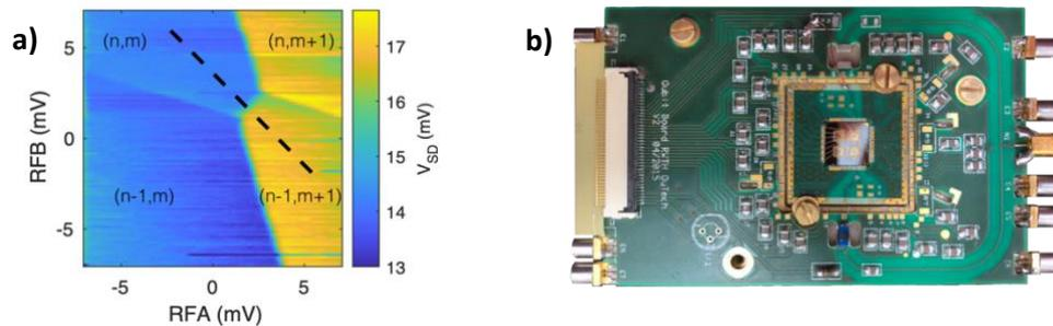
**Fig. 1 (a)** Stability diagram of a qubit acquired via charge sensing of an Asymmetric Sensing Dot (ASD). The ASD operates with a current bias and produces a much stronger signal than conventional readout sensors. **(b)** Picture of a quantum device sample (chip in the centre) with an integrated ASD. The chip is wire bonded to a printed circuit board, which is cooled down to 10 mK.
